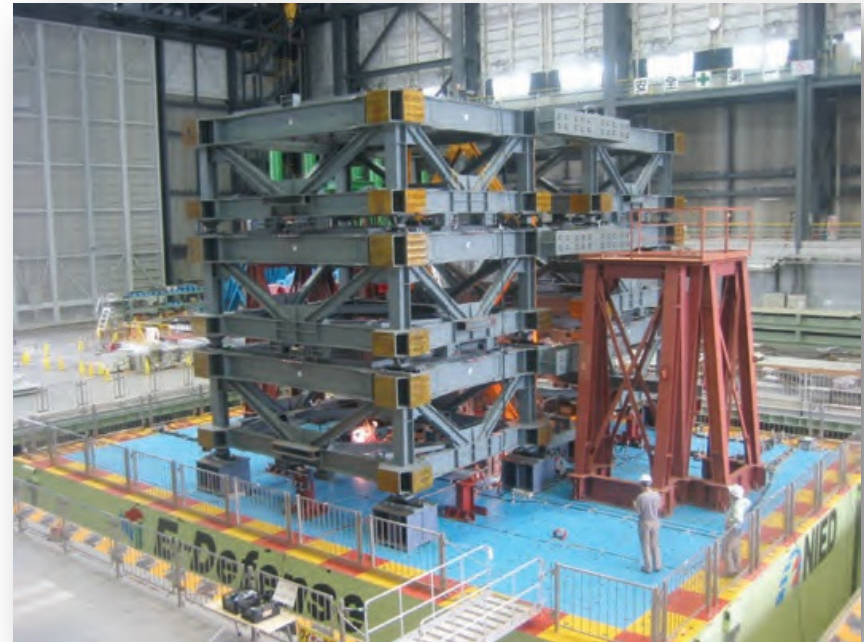
Multistory steel frame with energy dissipation
